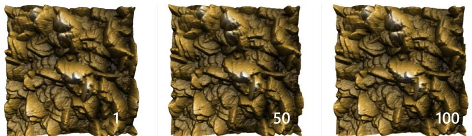
Consecutive unattended imaging of a TipCheck sample with CleanDrive excitation. After 100 images no noticeable change in the tip curvature could be observed. Image size:  $1\ \mu\text{m}$ . Z-height:  $90\ \text{nm}$ .
