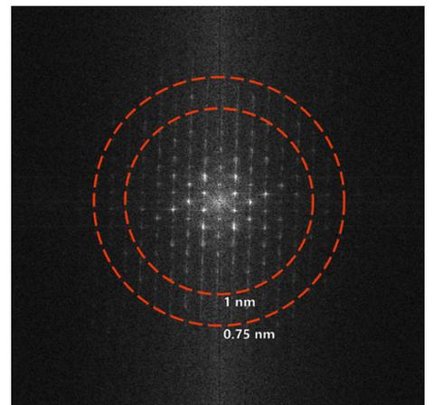
**Right:** 2D FFT spectrum of the image in the left. The dashed circles indicate resolution of 1 nm and 0.75 nm. The spectrum reveals diffraction peaks beyond the outer circle indicating a resolution better than 0.75 nm.
