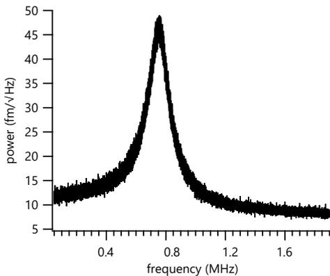
Thermal noise spectrum of a USF-F1.2-k7.3 cantilever in buffer solution. The thermal noise power spectrum reveals the broad resonance peak of the cantilever at approximately 750 kHz. The noise floor of the system can be clearly identified to be below 15 fm/√Hz, even before the resonance peak. At higher frequencies, the noise floor drops below 10 fm/√Hz.
