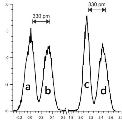
**Left:** topography image of an HOPG surface imaged in air. The surface shows different steps between different graphite layers. Image size: 500 nm. **Right:** height histogram of the HOPG surface. The spacing of two neighboring peaks in the histogram corresponds to 330 μm, the expected height of a graphite layer.
