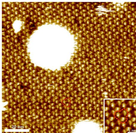
**Left:** high-resolution topography image of the cytoplasmic surface of purple membrane from *Halobacterium salinarum*. The topography clearly resolves the trimeric arrangement of bacteriorhodopsin (BR) proteins and substructures within the BR molecules. Inset: correlation average of BR trimers. The red dashed lines indicate a BR trimer.
