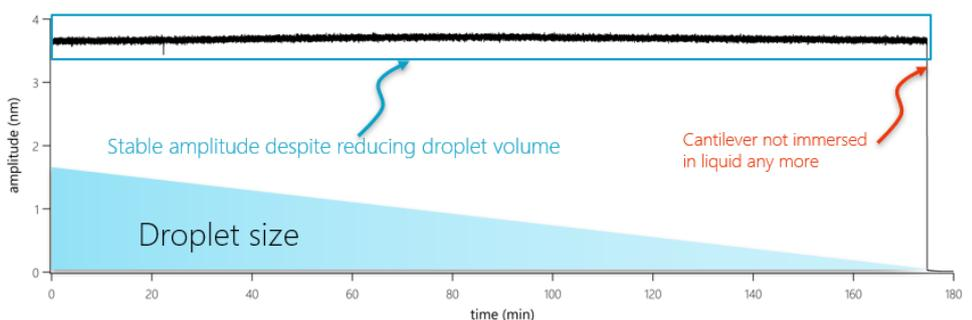
A cantilever immersed in a  $100\ \mu\text{l}$  buffer droplet was excited to an amplitude of  $3.6\ \text{nm}$ . The amplitude of the cantilever was observed while the buffer droplet was allowed to evaporate. Until the cantilever lost contact with the droplet, the amplitude of the cantilever did not change significantly. As the cantilever was released from the liquid, the amplitude suddenly dropped, as expected.
