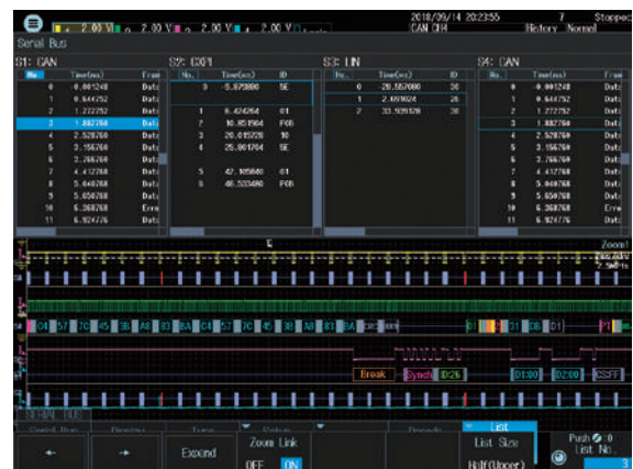
Four bus decode and list display
