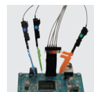
Example of logic probe connection
